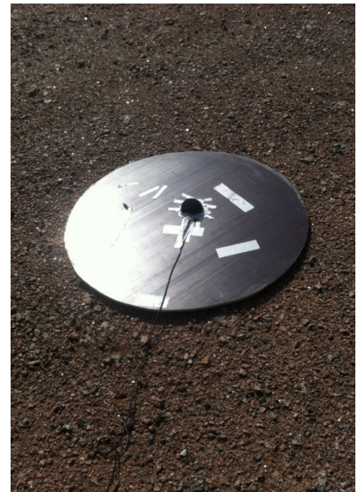
Figure 12 – Measurement board, turbine 4
