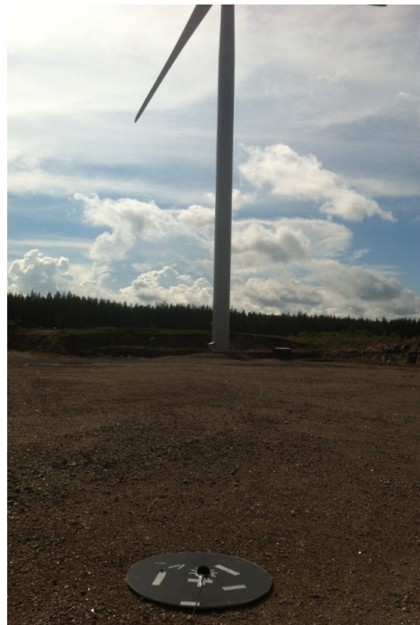
Figure 11 – Measurement position, Turbine 4
