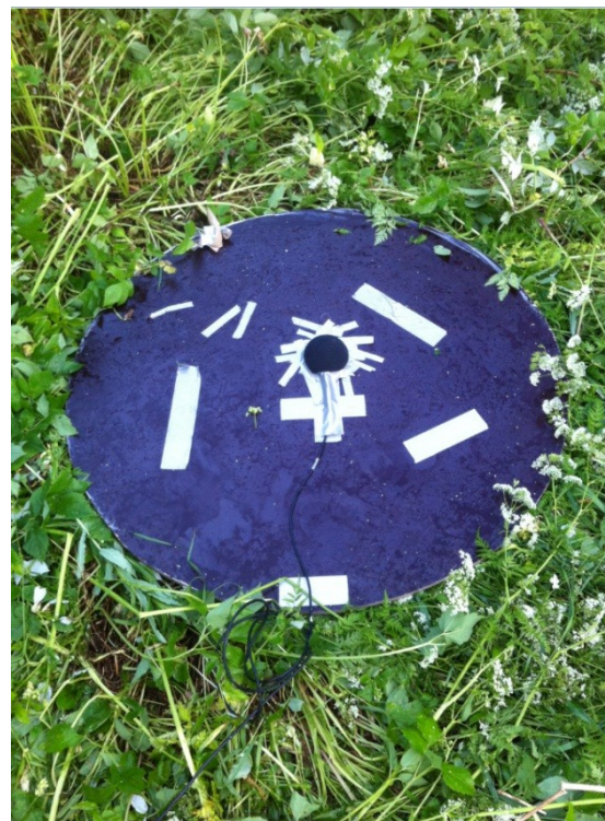
Figure 3 – Measurement board, turbine 1
