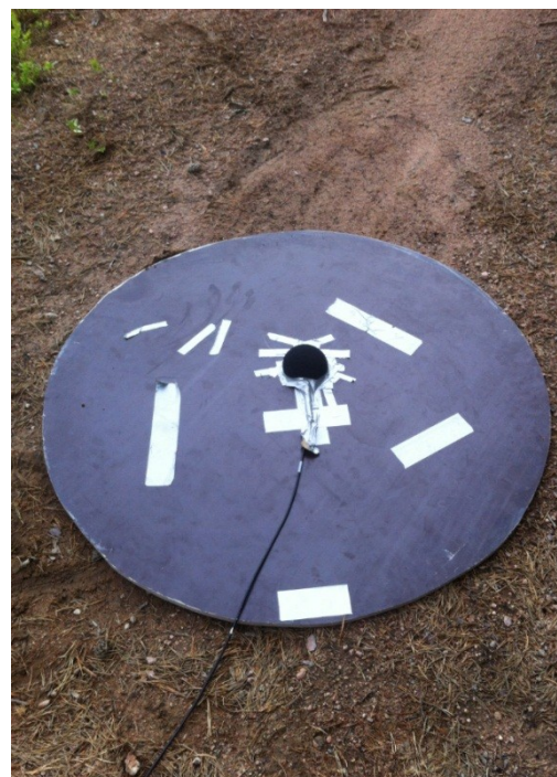
Figure 6 – Measurement board, turbine 2
